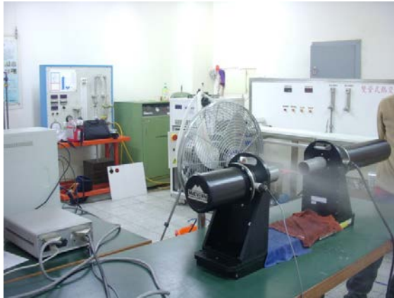
Fig. 4: Actual measurement of water spray particle size
